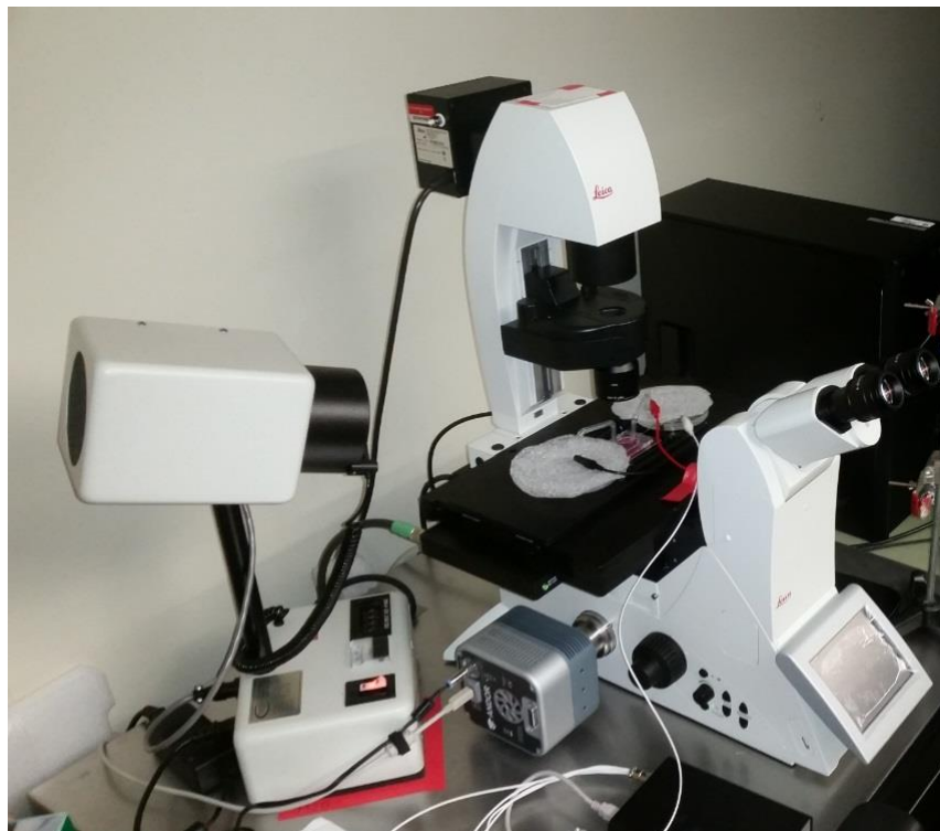
Figure 4. Experimental setup for imaging monolayers during electrotaxis
